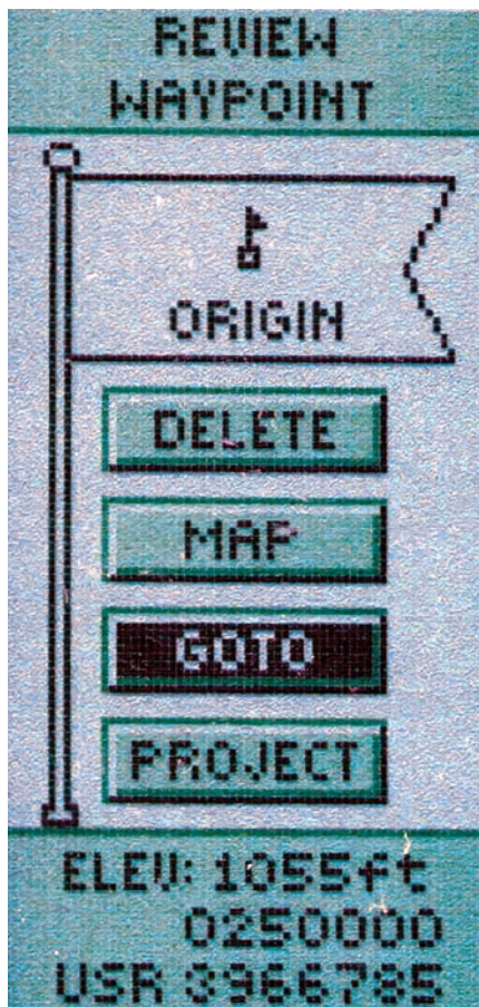
Figure 3 The waypoint at the Zone Origin displays the value of the False Northing when viewed in USER GRID format.
