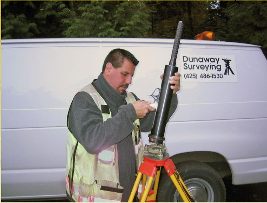
Spencer Hogue of Dunaway Surveying, Inc., in Bothell, WA, inserts a Thompson/Center Contender .45 caliber pistol into the tracer apparatus. This firearm is also capable of firing the .410 bore shotshell for first clearing the tree canopy.
