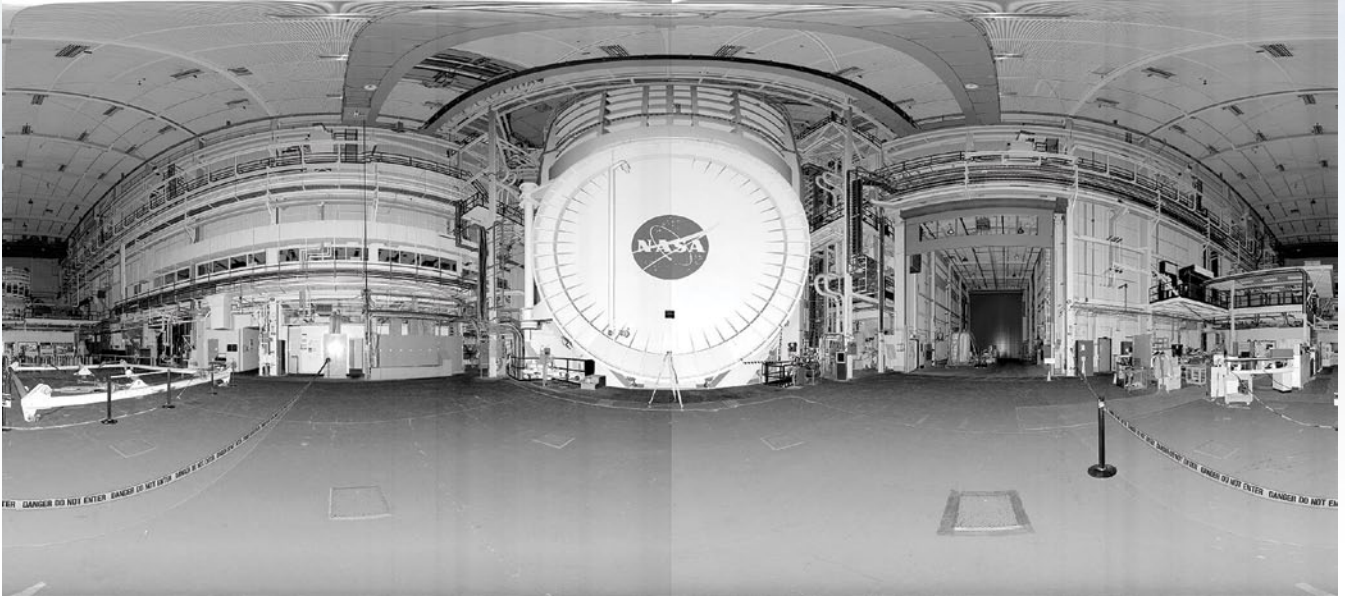
Point cloud data captured from the FARO LS 880 laser scanner. The photo-like image shown here was captured in FARO Cloud's Planar View. The point cloud is seen as a wrap around planar projection image.
