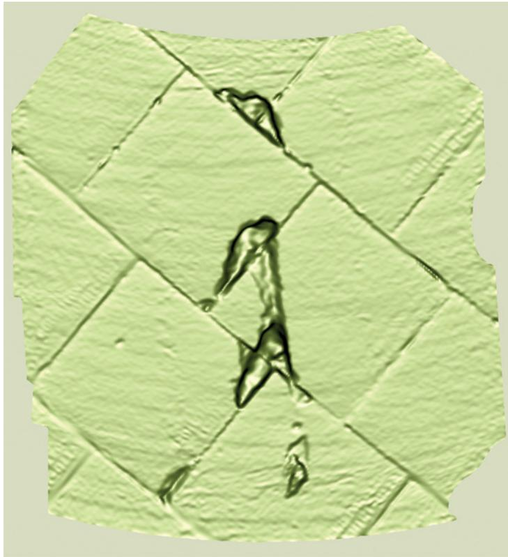
**Figure 4** Surface model of simulated tile damage created from point-cloud data by Raindrop Geomagic using Geomagic Studio. Image Courtesy Raindrop Geomagic, Inc.
