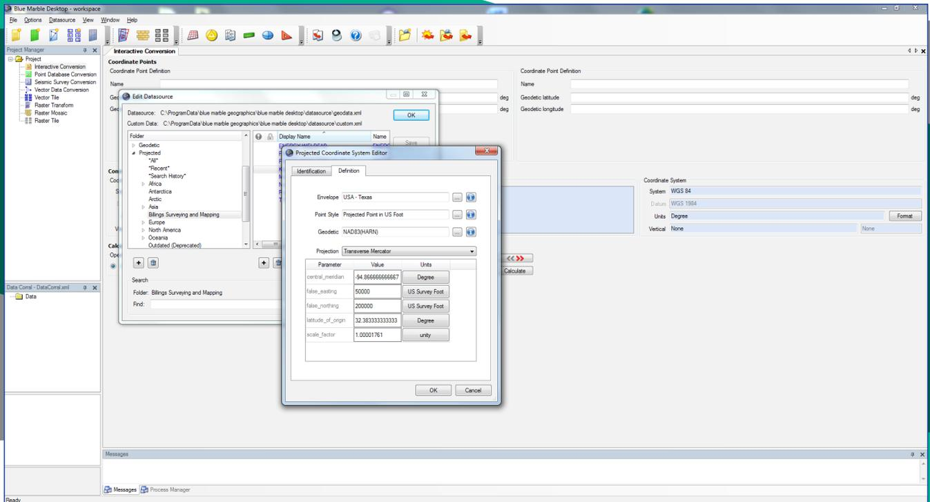
Blue Marble Geographic Calculator provides an incredible variety of tools for working with an infinite combination of datums and projections. Shown here, I've entered the parameters for a Low Distortion Projection for my home town. With these parameters established, I can transform numerous vector file types (such as .dwg, .dxf, and .dgn), numerous raster image file types (such as .sid, .jp2, .tif), or coordinate files to my new projection.
