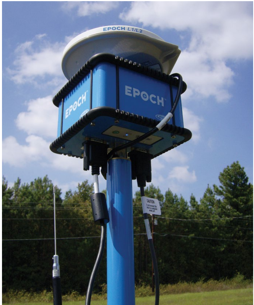
In this photo, the blue LED on the bottom of the Epoch 25 base indicates that the unit is on. Also visible are the two 9-pin serial plugs and the GPS antenna connection.
