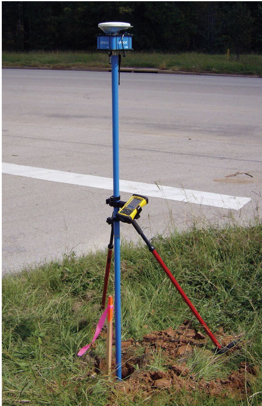
The rover is set up on an iron rod approximately two miles from the EPOCH 25 base station and is being controlled wirelessly via Bluetooth by the TDS Nomad using Survey Pro. The setup is compact, neatly arranged on the pole and well balanced.
