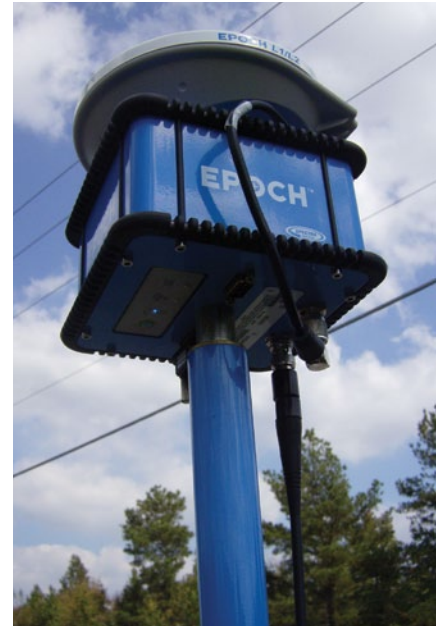
A close-up of the rover shows the “rubber ducky” UHF receiver antenna, the GPS antenna connection, an unused 9-pin serial port, the blue “on” LED light, and the Bluetooth adapter for wireless communication.
