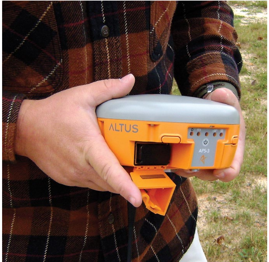
Two battery bays on the side are accessed by the press of a button, making it possible to change batteries with one hand.
