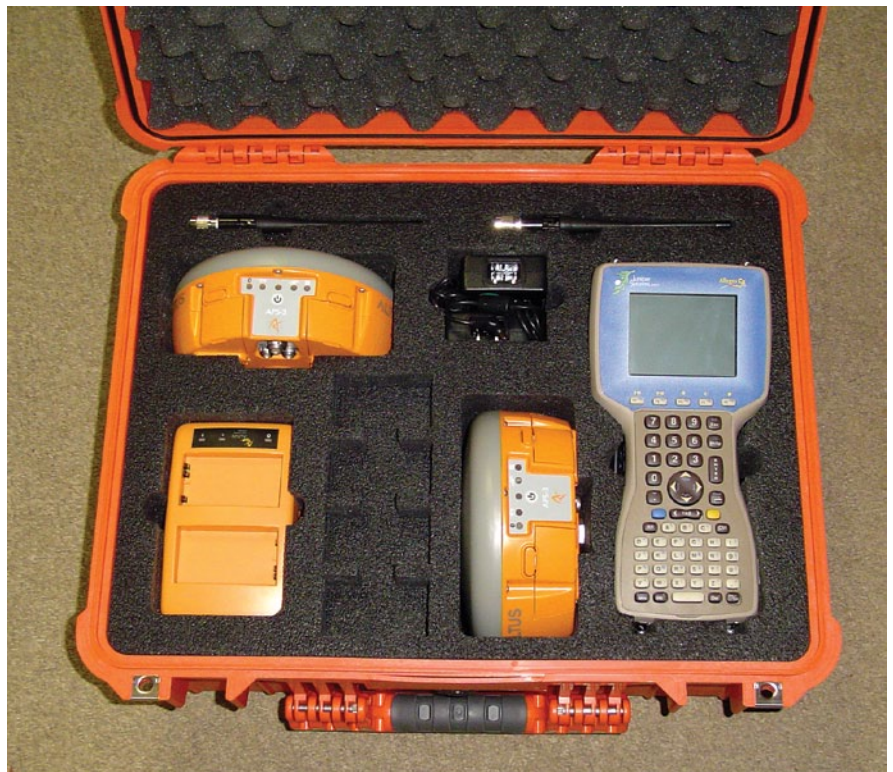
In one hand a solo operator can tote the entire APS-3 RTK system in a medium-sized Pelican case, and in the other hand tote a tripod, GPS pole, or that fourth cup of coffee.
