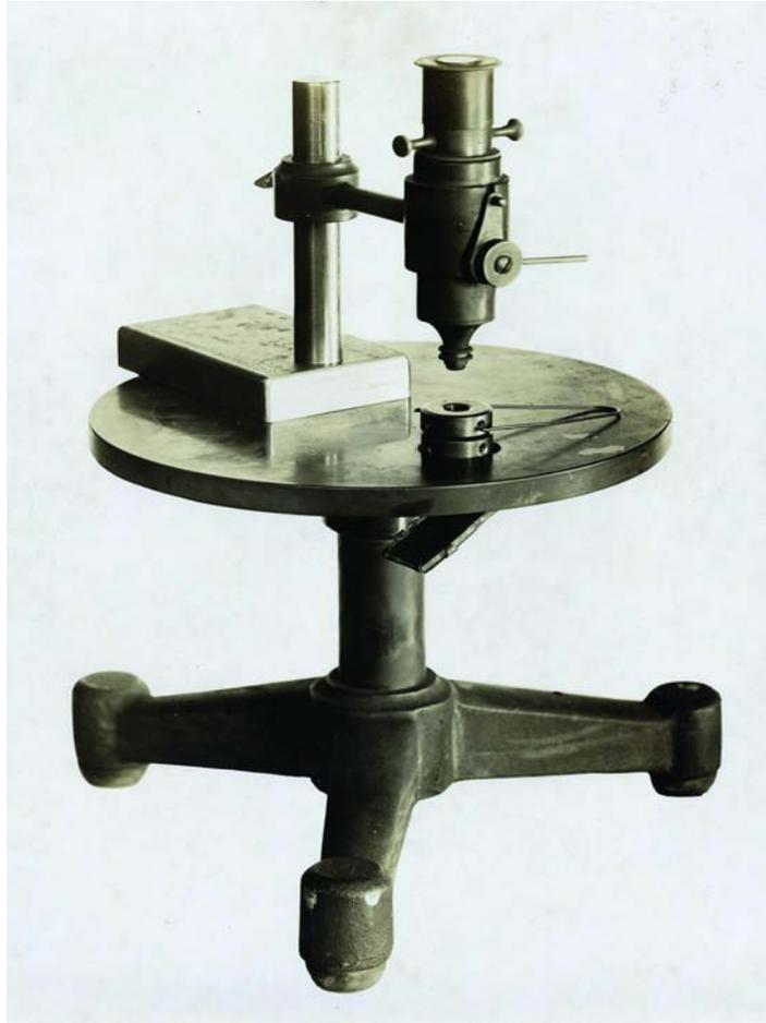
Ketteringham microscope for fixing spider silk in an instrument
