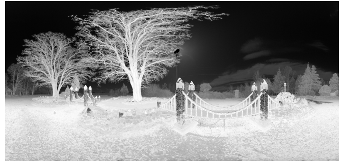
Laser scan data of the Peterson Rock Garden, showing two of the miniature bridges within the garden's landscape. Image courtesy of Restore Oregon, who listed the site on Oregon's "Most Endangered Places List" and ToPa 3D, Inc., who documented the site with 3D laser scanning and panoramic photography.
