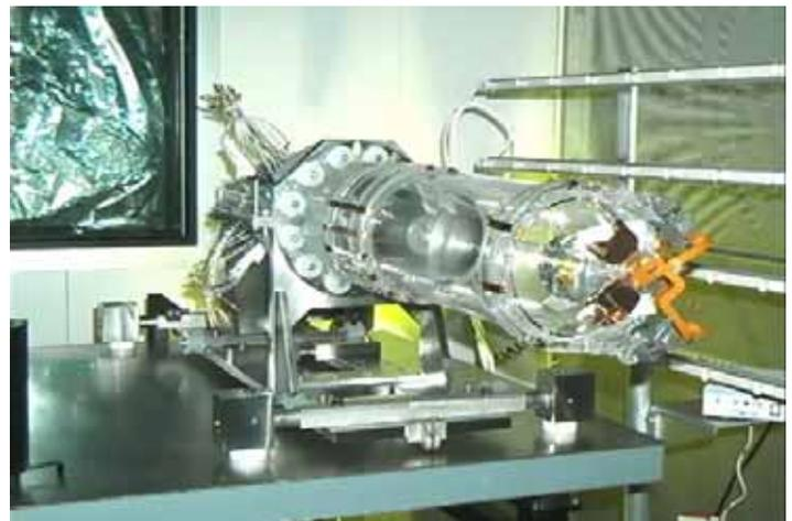
*The telescope (front) is shown bonded to the integrated quartz block. The gyroscope lines (visible in the back) protrude from the quartz block.*
