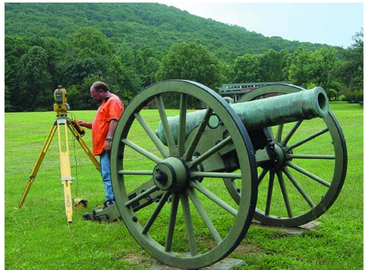
Scott Holcombe of GeoSurvey, Ltd., operates a Topcon AP-L1A robotic station while collecting data for the base map.
